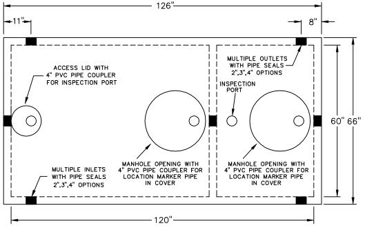
SPECIFICATIONS SEPTECH MIN 1750 GALLON 2-COMPARTMENT GREASE TRAP NJ1750GT-2C
