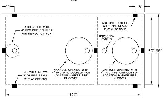
SPECIFICATIONS | SEPTECH<sup>™</sup> NJ 1750 GALLON 2-COMPARTMENT SEPTIC TANK
