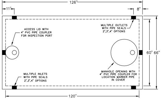
SPECIFICATIONS SEPTECH ™ NJ 2000 GALLON 1-COMPARTMENT GREASE TRAP NJ2000GT
